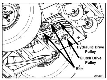
Pump/Motor Belt Removal Figure 4-13
